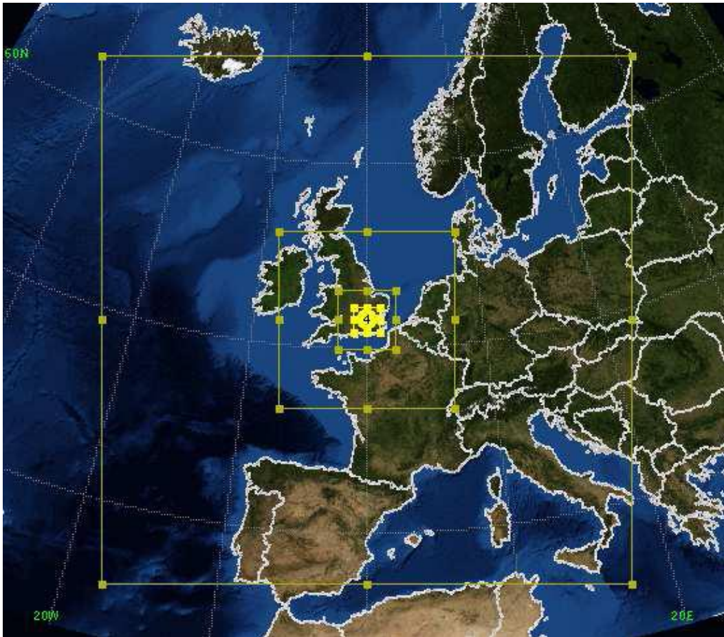
Figure 4: Example of nested grid in the WRF model, gradually nesting in on the London Metropolitan Area. The outer domain has a grid size of 81 km, the second domain has 27 km grid size, the third 9 km, and the fourth 3 km grid size. The innermost domain with 1 km grid size is not shown. Source: WRF Domain Wizard.
