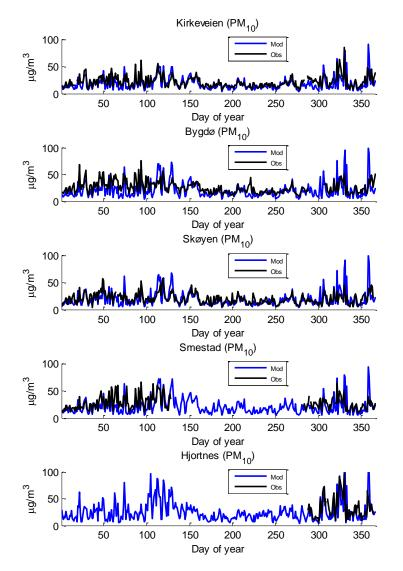
Figure 14: Daily mean PM<sub>10</sub> concentrations at 9 monitoring sites in Oslo for the calendar year 2008. Blue is the model (including regional background) and black is the observations. The lower right plot indicates the regional background concentrations.
