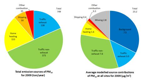
Figure 18: Total emissions of  $PM_{10}$  per year in tons (left) and modelled source contribution of mean  $PM_{10}$  concentrations for all the measurement sites. 'Missing' is the observed minus total modelled concentrations.
