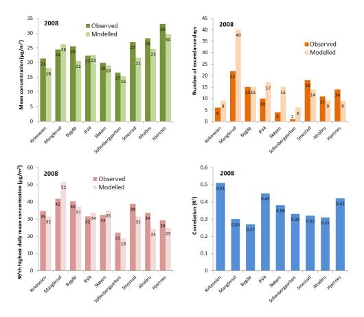
Figure 16: Calculated mean concentrations (left) and number of exceedance days, days with daily mean concentrations of  $PM_{10} > 50 \ \mu g/m^3$ , (right) for the year 2008 at 9 monitoring stations in Oslo. Model values presented are concurrent with available monitoring data.
