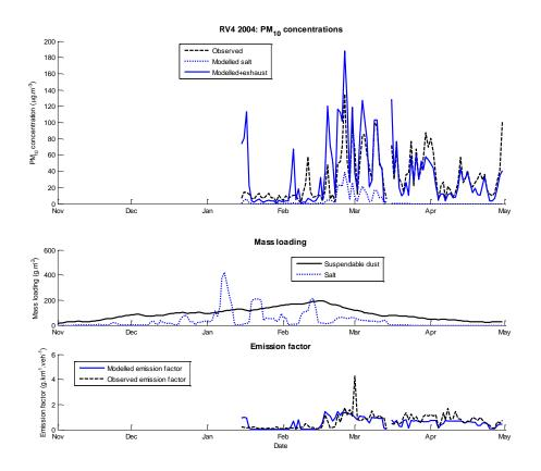
Figure 3: Results of the model application at RV4 for the period November 2003 to April 2004. Top: Daily mean modelled and observed concentrations of PM<sub>10</sub> including salt contribution. Middle: Surface mass loading of suspendable dust and salt. Bottom: Effective emission factor for PM<sub>10</sub> calculated by the model and derived from observations.
