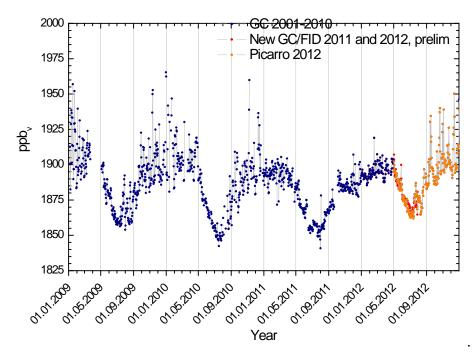
Figure 56: Daily mean of methane measured with the old GC (2001-2010), new GC-FID in 2011 -> and a new Picarro (Cavity Ring-Down Spectrometer) run in parallel in 2012.
