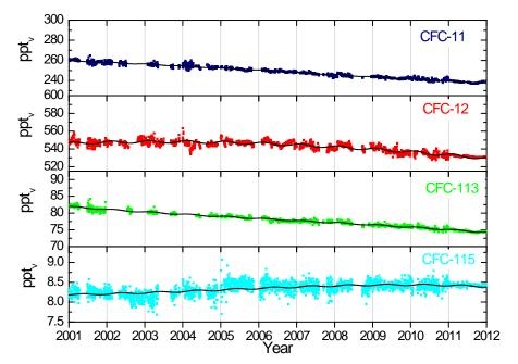
Figure 20: Daily averaged mixing ratios of the monitored CFCs: CFC-11 (dark blue), CFC-12 (red), CFC-113 (green) and CFC-115 (light blue) for the period 2001-2011 at the Zeppelin observatory. The solid lines are modelled background mixing ratio.
