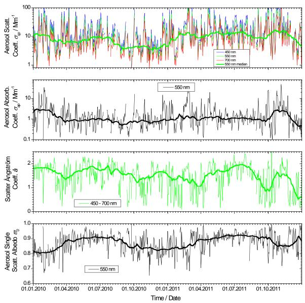
Figure 37: Aerosol optical properties daily means measured in 2010 and 2011 at Birkenes. Top panel: aerosol scattering coefficient  $\sigma_{sp}$  at 450, 550, and 700 nm wavelength. Second panel: aerosol absorption coefficient  $\sigma_{ap}$  at 550 nm wavelength. The third and forth panels: the scattering Ångström coefficient  $\mathring{a}_{sp}$  and the single scattering albedo  $\varpi^0$  as derived properties, respectively.
