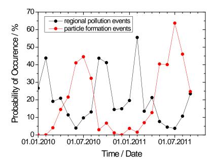
Figure 41: Frequency of occurrence of influence by local or regional combustion, as well as occurrence of new particle formation in Birkenes in 2010 as determined by combined analysis of particle number size distribution and single scattering albedo.
