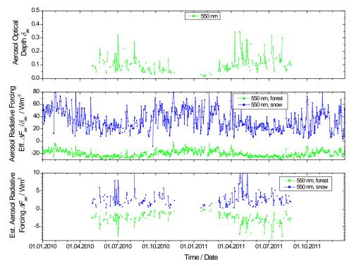
Figure 38: 2010 and 2011 time series aerosol optical depth (AOD) at 550 nm wavelength above Birkenes (upper panel), as well as the radiative forcing efficiency  $\Delta F_{ae}/\delta$  (middle panel) and the estimated local, instantaneous, solar aerosol radiative forcing  $\Delta F_{ae}$ , the latter two for surface albedo for forest and snow, respectively.
