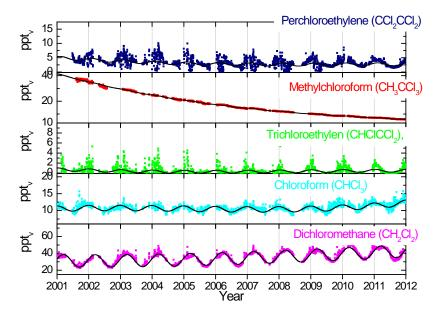
Figure 28: Daily average concentrations chlorinated hydrocarbons: From the upper panel: perchloroethylene (dark blue) methylchloroform (red), trichloroethylen (green), chloroform (light blue) and dichloromethane (pink) for the period 2001-2011 at the Zeppelin observatory. The solid lines are the modelled background mixing ratio.
