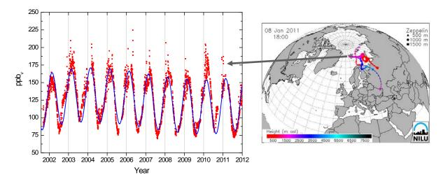
Figure 18: Observations of carbon monoxide (CO) from the September 2001 to 31.12.2010 at the Zeppelin observatory. Red dots: daily averaged observed mixing ratios. The solid line is the modelled background mixing ratio. The maximum value in 2011 is caused by transport of pollution from North west Russia.
