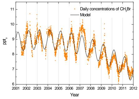
Figure 15: Observations of methyl bromide,  $CH_3Br$ , for the period 2001-2011 at the Zeppelin observatory. Dots: daily averages mixing ratios from the observations, solid line: modelled background mixing ratio.
