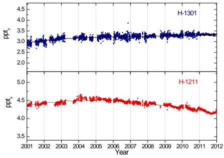
Figure 26: Daily average concentrations of the monitored halons: H-1301 (blue in the upper panel) and H-1211<sup>5</sup> (Red in the lower panel) for the period 2001-2011 at the Zeppelin observatory. The solid lines are modelled background mixing ratio.
