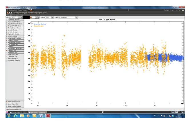
Figure 53: Measurements of CFC-115 at Zeppelin Observatory. The measurement precision improves when using results from the Medusa-GCMS (in blue) compared to the ADS-GCMS (in yellow).
