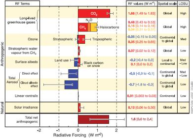
Figure 1: Global-average radiative forcing (RF) estimates for important anthropogenic agents and mechanisms together with the typical spatial scale of the forcing and the assessed level of scientific understanding (LOSU).
