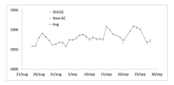
Figure 54: Comparison of old and new measurements of methane at Zeppelin.
