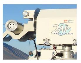
PFR-GAW - Precision Filter Radiometer
