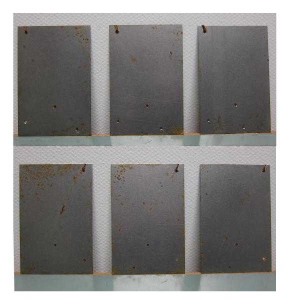
Figure 11B: Samples 2D MEA after exposure (Swedish DC01 steel, three samples, both sides).
