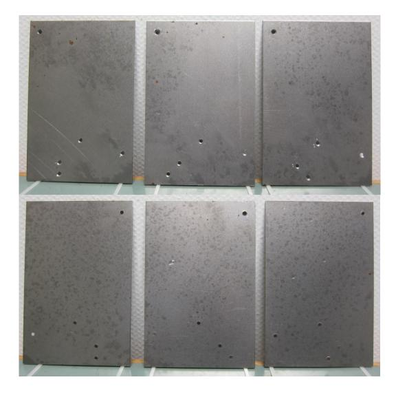
Figure 12B: Samples 4B MEA after exposure (Swedish DC01 steel, three samples, both sides).
