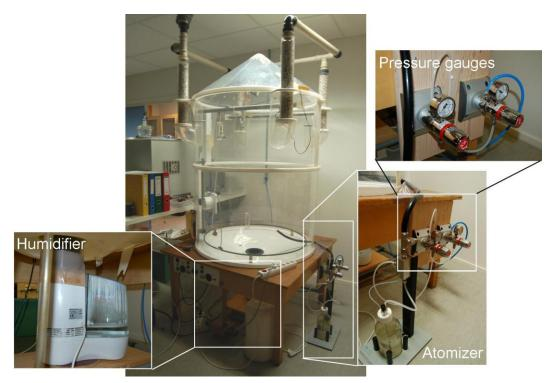
*Figure 3:* The fog and aerosol chamber.
