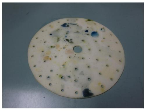
*Figure 15:* Dissolved copper in DEA solution of high concentration having run off a copper sample.
