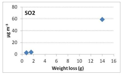
*Figure 30:* Correlation of annual average values for the SO<sub>2</sub> concentration, and carbon steel corrosion.
