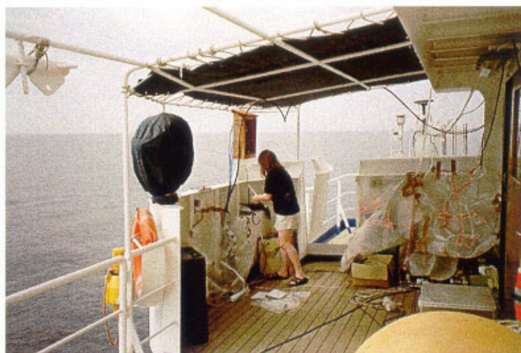
Figure 11: Changing denuders in the sampling box on the upper deck.
