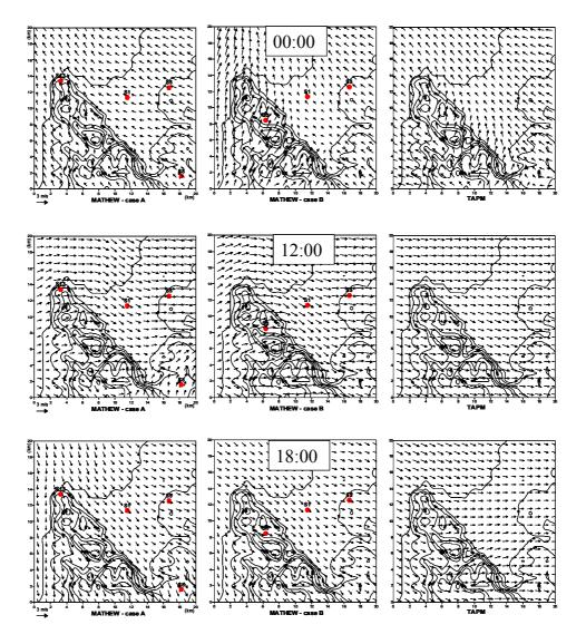
Figure 14: Wind fields produced by MATHEW for Case A (left), Case B (centre).
