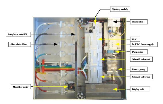
Figure A. 1: Instrument layout (lid removed).
