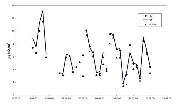
*Figure 5: Comparison of NO*<sub>2</sub> *measurements using NILU-FK, SS2000 and monitor*
