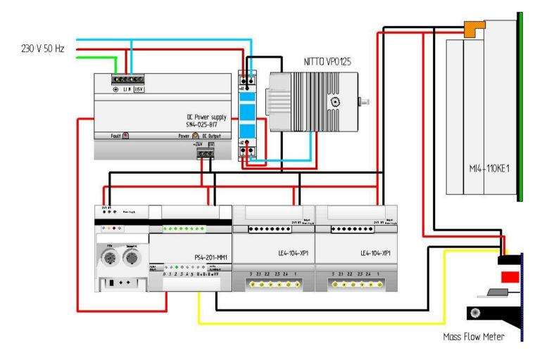
Figure C.1: Wiring diagram for NILU SS2000.
