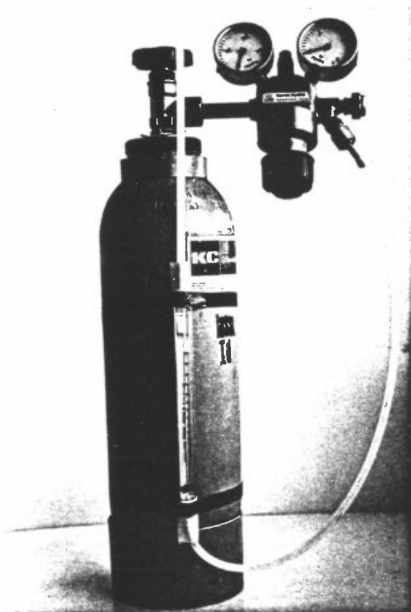
Figure 2: \text{SF}_6 cylinder and gas flow meter.
