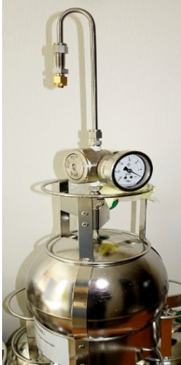
Figure 3 NILUs 3 litre canisters with critical orifice and pressure manometer
