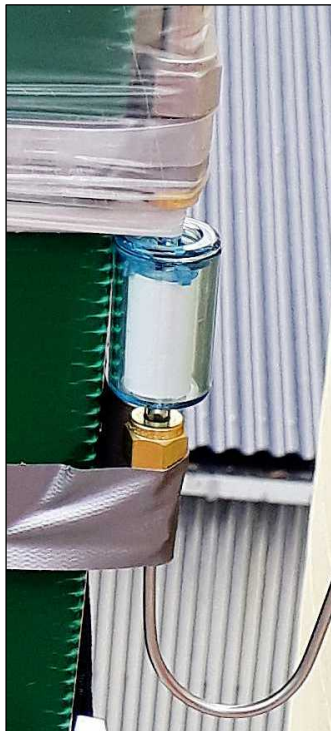
Figure 5 The 2 photos above: Particle filter after 30 days of sampling – one without any signs of water clogging – the other filled with water.
