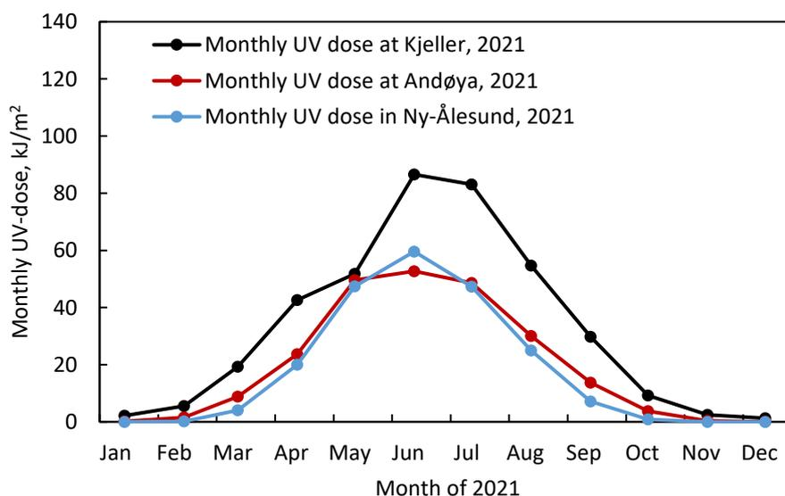
Figure 18: Monthly integrated UV doses (in kJ/m<sup>2</sup>) in 2021 measured with the GUV instruments located at Kjeller, Andøya and in Ny-Ålesund.
