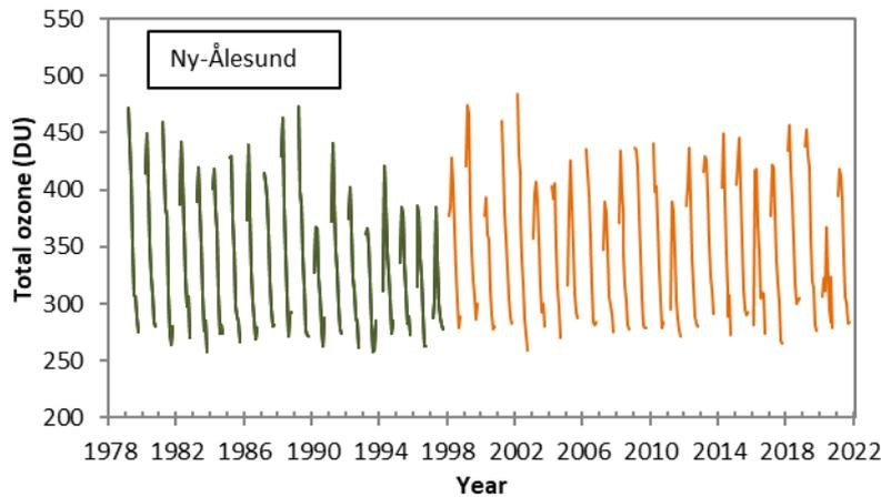
Figure 6a: Time series of monthly mean total ozone at Ny-Ålesund 1979–2021. The green line represents total ozone data from satellite, whereas the orange line represents measurements from ground-based instruments.
