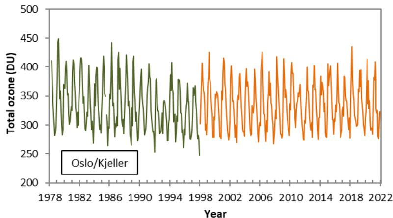
Figure 4a: Time series of monthly mean total ozone in Oslo and at Kjeller 1979–2021. The green line represents measurements performed with the Dobson instrument, whereas the orange line represents Brewer measurements.
