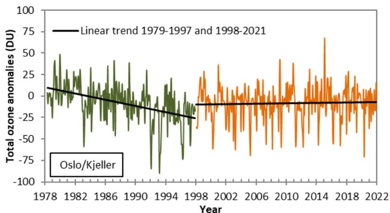
Figure 4b: Variation in total ozone over Oslo/Kjeller for the period 1979–2021 after the seasonal variations have been removed. The green line represents measurements performed with the Dobson instrument, whereas the orange line represents Brewer measurements. Trend lines are marked as black lines.
