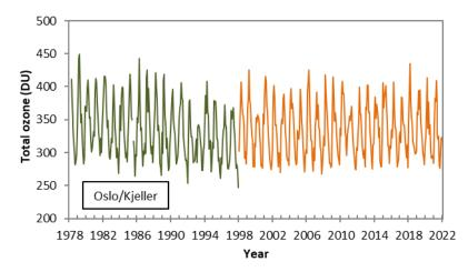
Figure 4a: Time series of monthly mean total ozone in Oslo and at Kjeller 1979-2021. The green line represents measurements performed with the Dobson instrument, whereas the orange line represents Brewer measurements.
