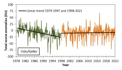
Figure 4b: Variation in total ozone over Oslo/Kjeller for the period 1979–2021 after the seasonal variations have been removed. The green line represents measurements performed with the Dobson instrument, whereas the orange line represents Brewer measurements. Trend lines are marked as black lines.
