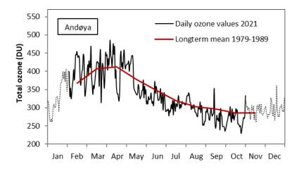
Figure 2a: Daily total ozone values measured at ALOMAR, Andøya, in 2021 by the Brewer and GUV instruments (black curve). The red line is the long-term monthly mean values from 1979-1989. The dotted line represents GOME2 satellite measurements.
