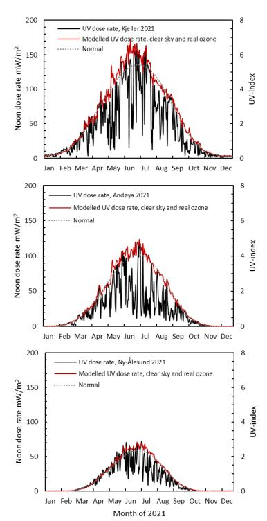
Figure 16: Hourly averaged UV dose rate measured at local noon (± 0.5 hour) in 2021. Upper panel: Kjeller. Middle panel: Andøya. Lower panel: Nv-Ålesund.
