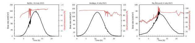
Figure 17: UV dose rates (left axis, black curves) and cloud transmission (right axis, red curves) during the days of maximum UVI at Kjeller (left panel), Andøya (middle panel) and Ny-Ålesund (right panel) in 2021. A cloud transmission of 100% represents clear sky conditions, whereas cloud transmissions of 20-30% represent heavy clouds.
