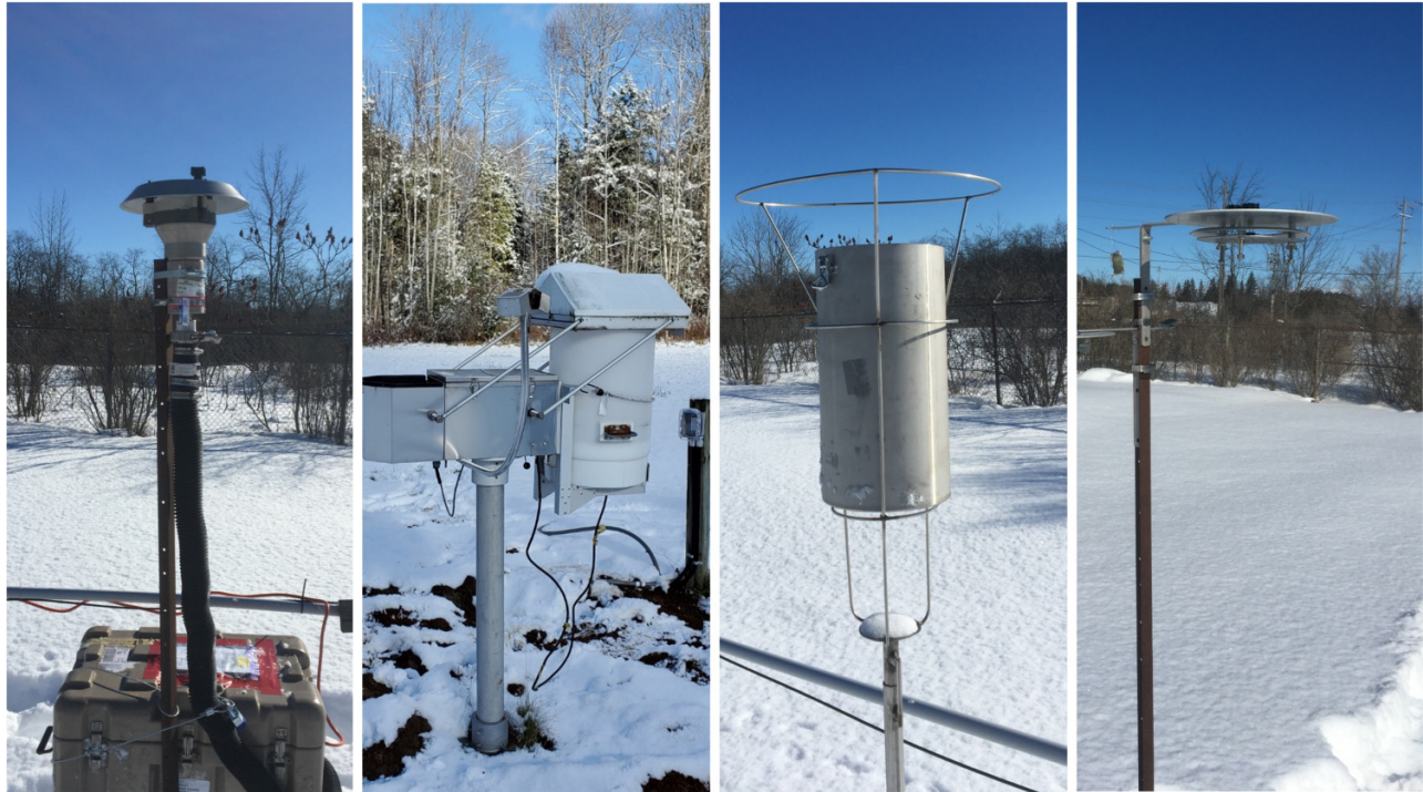
Fig. 2. Sampling equipment for atmospheric microplastics: photographs showing (from left to right) active air sampling (with sampling head), wet deposition only sampling, NILU bulk deposition collector, and passive air sampling (including moss bags).
