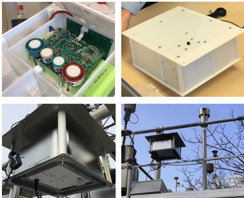
Fig. 1 AirSensEUR sensor systems: (top left) chemical shield with gas sensors; (top right) sensor box with sampling inlet of OPC-N3 on top; (bottom left) sensor box in outdoor enclosure with gas sensors and PMS5003 sensor inlet and (bottom right) sensor box installed at Air Quality Monitoring Stations.
