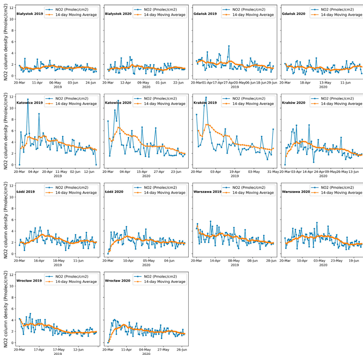
FIGURE 3 TROPOMI NO 2 daily variations (blue) and a 14-day moving average (orange) in selected Polish cities (locations in Figure 1) between 20 March and 30 June of 2019 and 2020.
