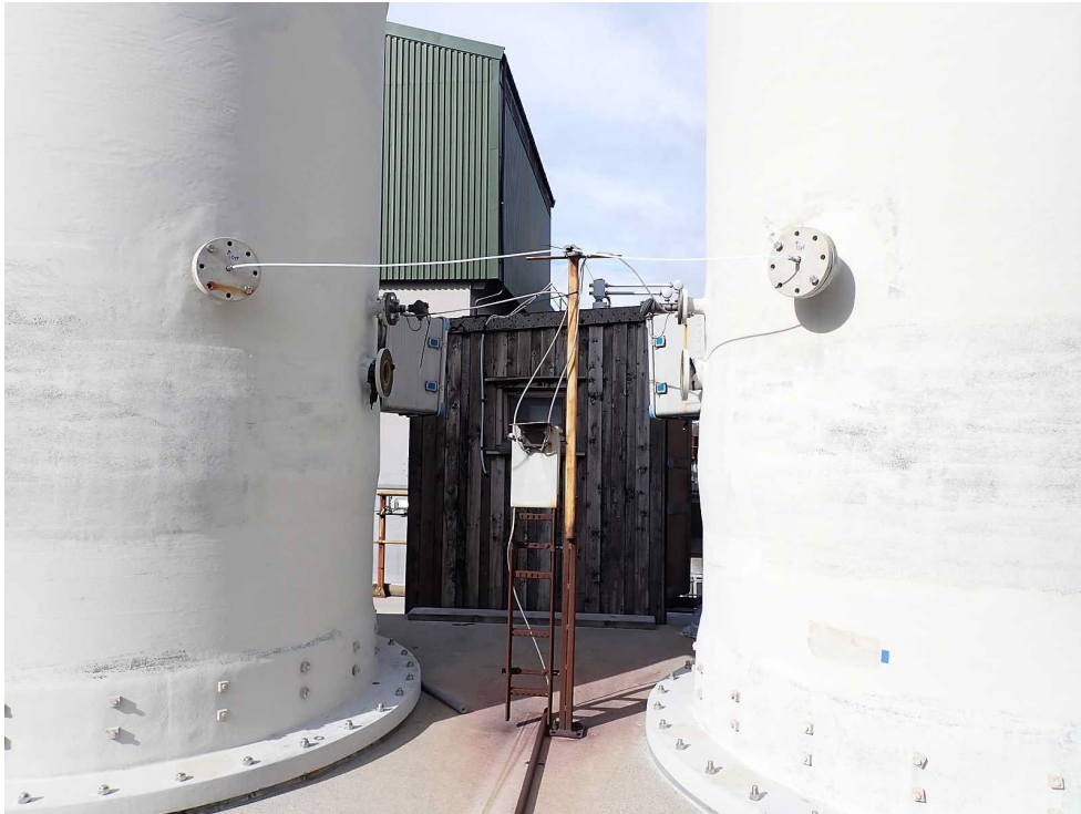
Figure 3: The samples taken with a down facing inlet tube inside the stack in order to prevent water clogging. CSIROs four canisters with pressure logger were used during the campaign at Mosjøen. For each of the two chimneys one inlet line was split into two different flow restrictors (CSIRO's, 0.004" tubing and NILU's critical orifice ) after passing a particle filter and HF-scrubber.
