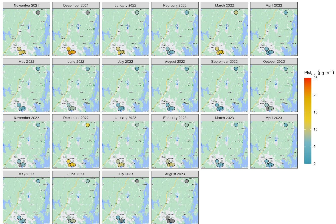
Figure A4: Spatial distribution of monthly PM_{2.5} for the Sandefjord air quality sensors. Warm/cold colors are for high/low PM_{2.5} concentrations. Missing data cases are drawn with grey circles. A monthly average is calculated assuming data completeness of 75% (more than 75% of available daily measurements per month).
