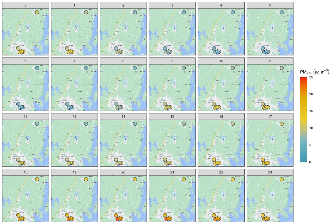
Figure A6: Spatial distribution of diurnal PM_{2.5} in winter (DJF) for the Sandefjord air quality sensors. Warm/cold colors are for high/low PM_{2.5} concentrations. Missing data cases are drawn with grey circles.
